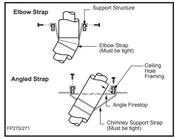
Fig. 18 Attach straps to a structural framing member.
